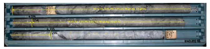
Figure 4 Massive sulphide mineralisation in drill core from hole BRD018 253.0m-255.5m.
