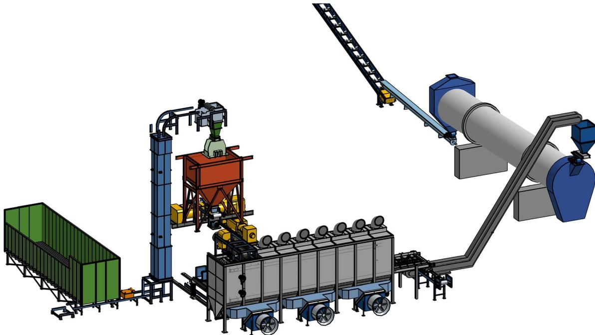
**Above:** Diagram 2 showing the direct feed concept of conditioned COLDry pellets to the pyrolysis kiln.
