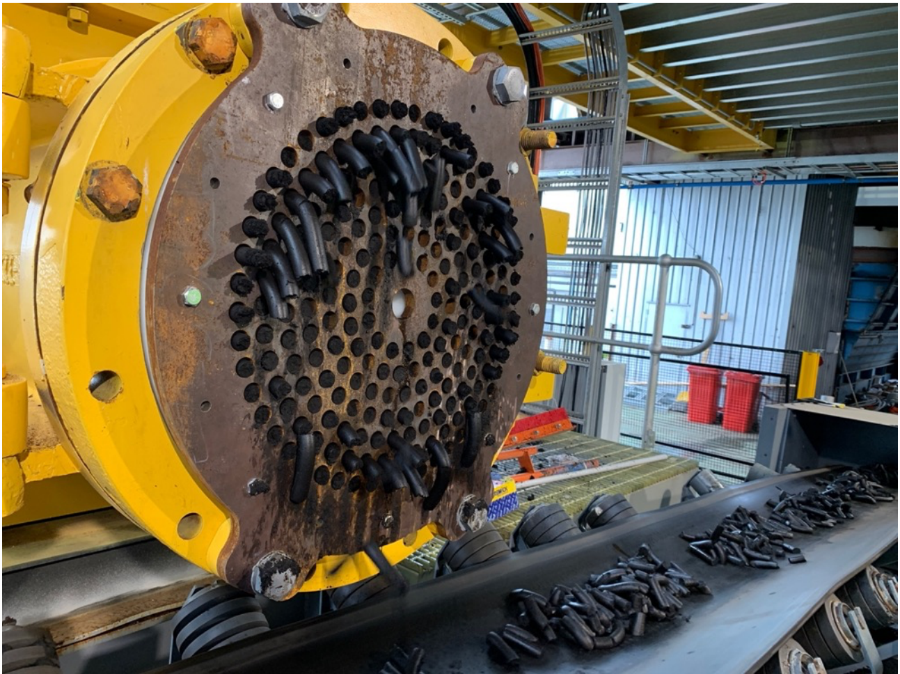
Photo (above): successful plasticisation and extraction of Yallourn lignite achieved. Subsequent drying of sample pellets confirmed the drying rate and compressive strength of the finished pellet were accomplished.
