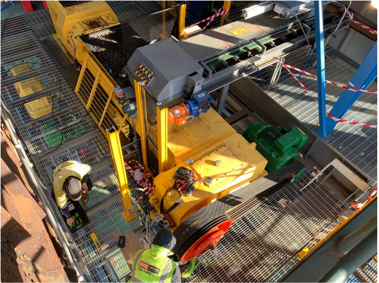
Photo (above): the weigh belt conveys the crushed lignite to the mixer. The mixer adds a specific amount of water to the incoming lignite prior to progressing to the pugmill.
