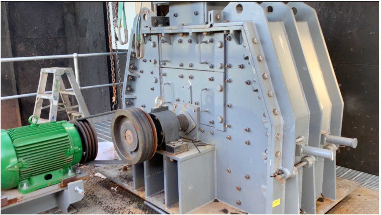
Photo (above): the hammer mill takes the as-mined lignite and reduces the average particle size prior to entering the surge hopper.
