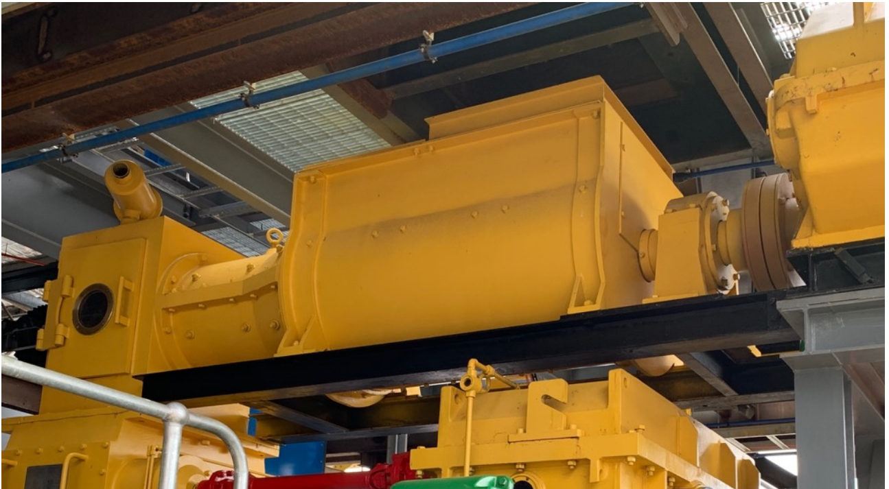
Photo (above): the pugmill provides a high level of shear to the lignite paste, further reducing the particle size, plasticising the material and initiating lignite densification prior to progressing to the extruder.
