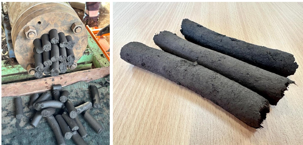
Photos (above): Successful bench scale extrusion of biomass-lignite COLDry pellets (left) and dried COLDry pellets made using Yallourn, Loy Yang and Maddingley lignite combined with waste hardwood saw dust (right).
