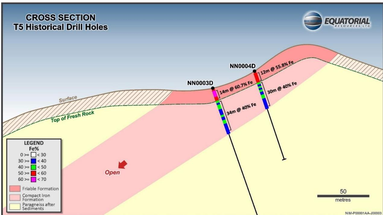
Figure 3 – Cross Section at T5 of Historical Drill Holes Showing High-Grade Cap
