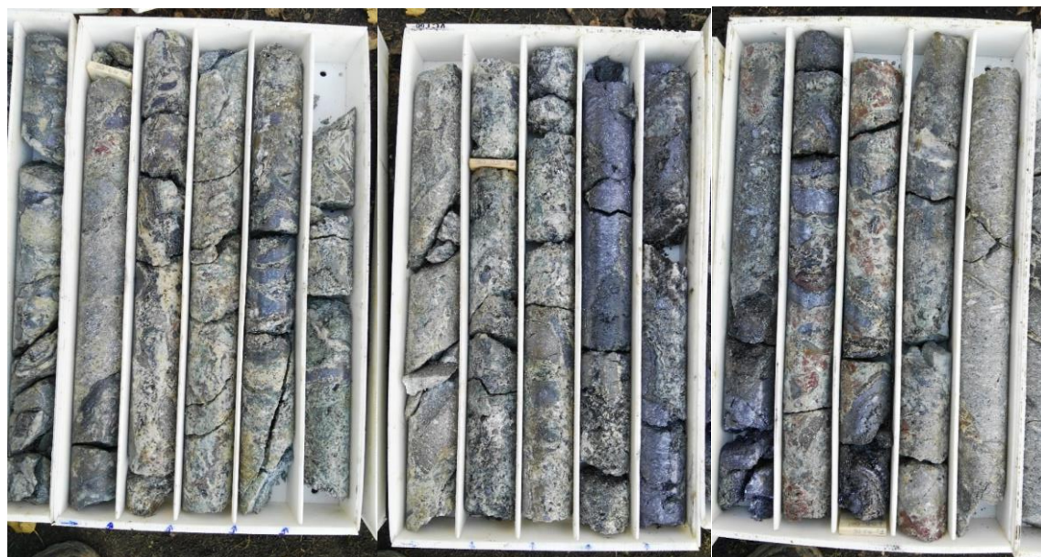
Photo 2. Drill Hole LDD 001 drill core at 46 to 55 metres depth showing strong galena rich, quartz vein and breccia mineralisation
