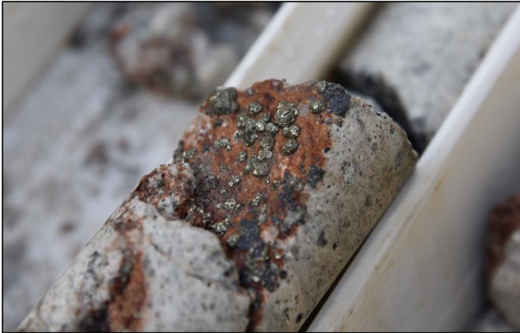
Photo 1. Example of sulphide rich quartz vein mineralization (black sulphide mineral interpreted to potentially correspond to a Ag sulfosalt mineral (acanthite \text{Ag}_2\text{S} or polybasite [(\text{Ag,Cu})_6(\text{Sb,As})_2\text{S}_7][\text{Ag}_9\text{CuS}_4] )
