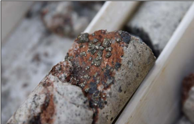
Photo 3. Example of sulphide rich quartz vein mineralization (black sulphide mineral interpreted to potentially correspond to a Ag sulfosalt mineral (acanthite Ag_2S or polybasite [(Ag,Cu)_6(Sb,As)_2S_7][Ag_9CuS_4] )
