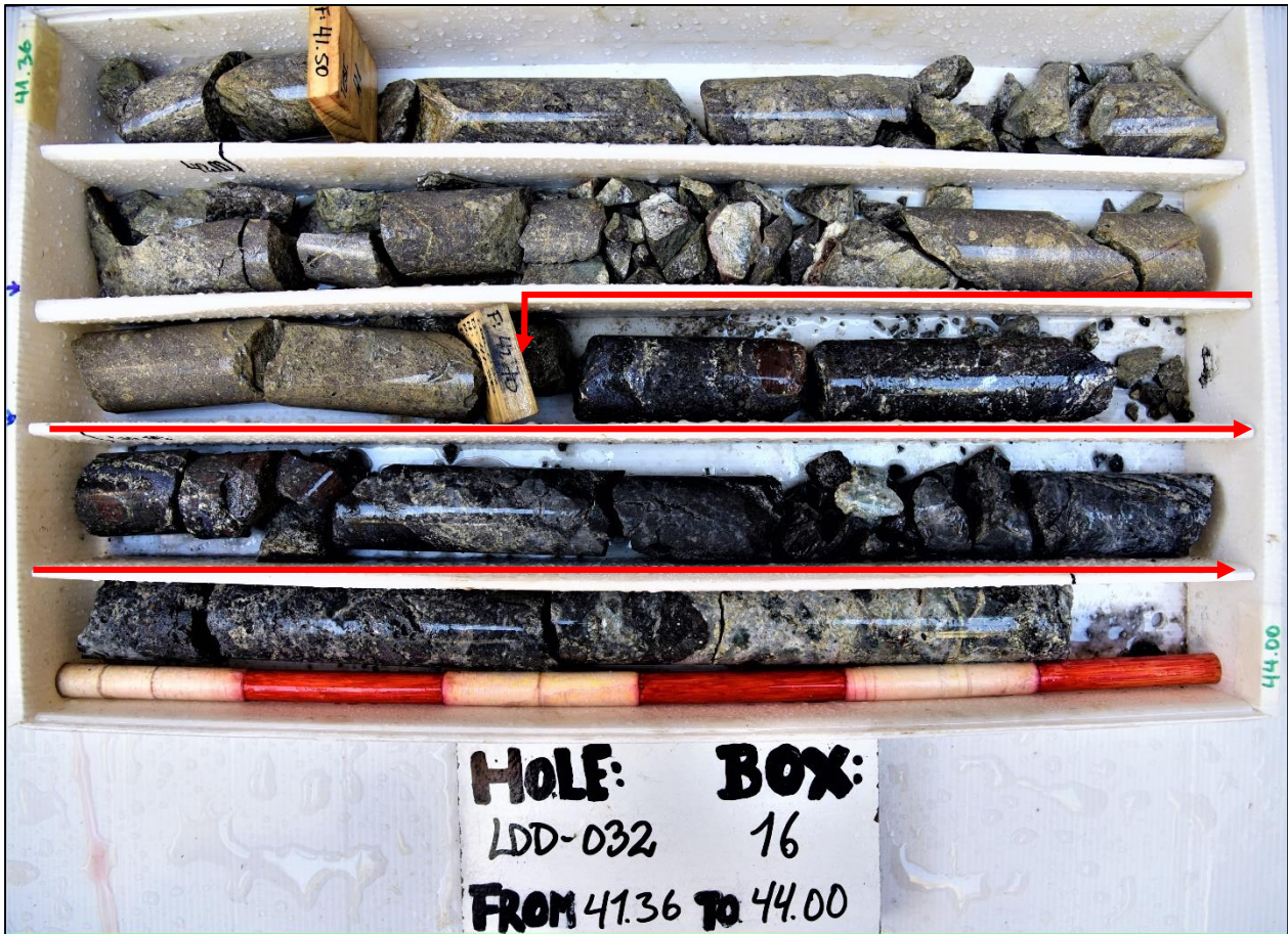
Photo 3 & 4. LDD-032 Visual high grade Ag, Pb, Zn vein-breccia (42.7- 45.5m)
