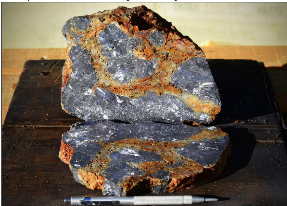
Photo 3. Float specimen with massive argentiferous galena found in Phase II drill area
