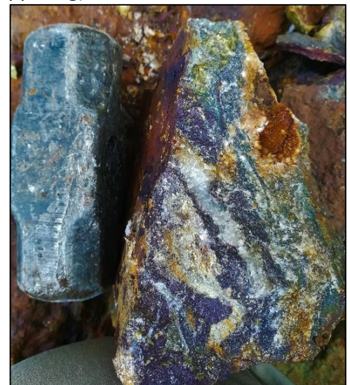
Image 2. Outcropping high grade copper mineralisation hosted in quartz veining (4.34% Cu, 12.5 ppm Ag)
