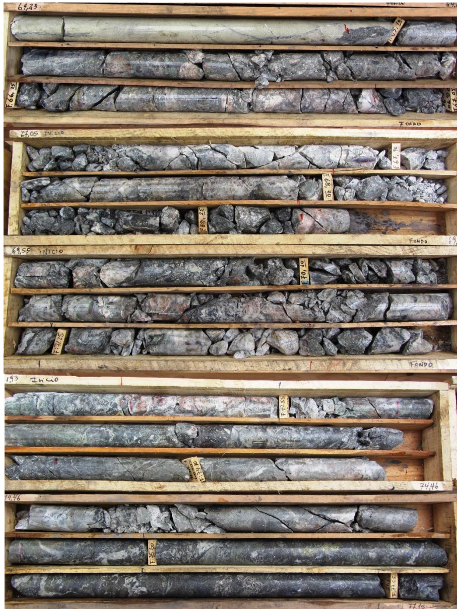
Photo 1. Hole CBD007: 65.05-77.15m interval: Saccharoidal to chalcedonic quartz veining with brecciated vein clasts cemented by black pyrite- Sb-Zn-As-Mo rich chalcedonic quartz
