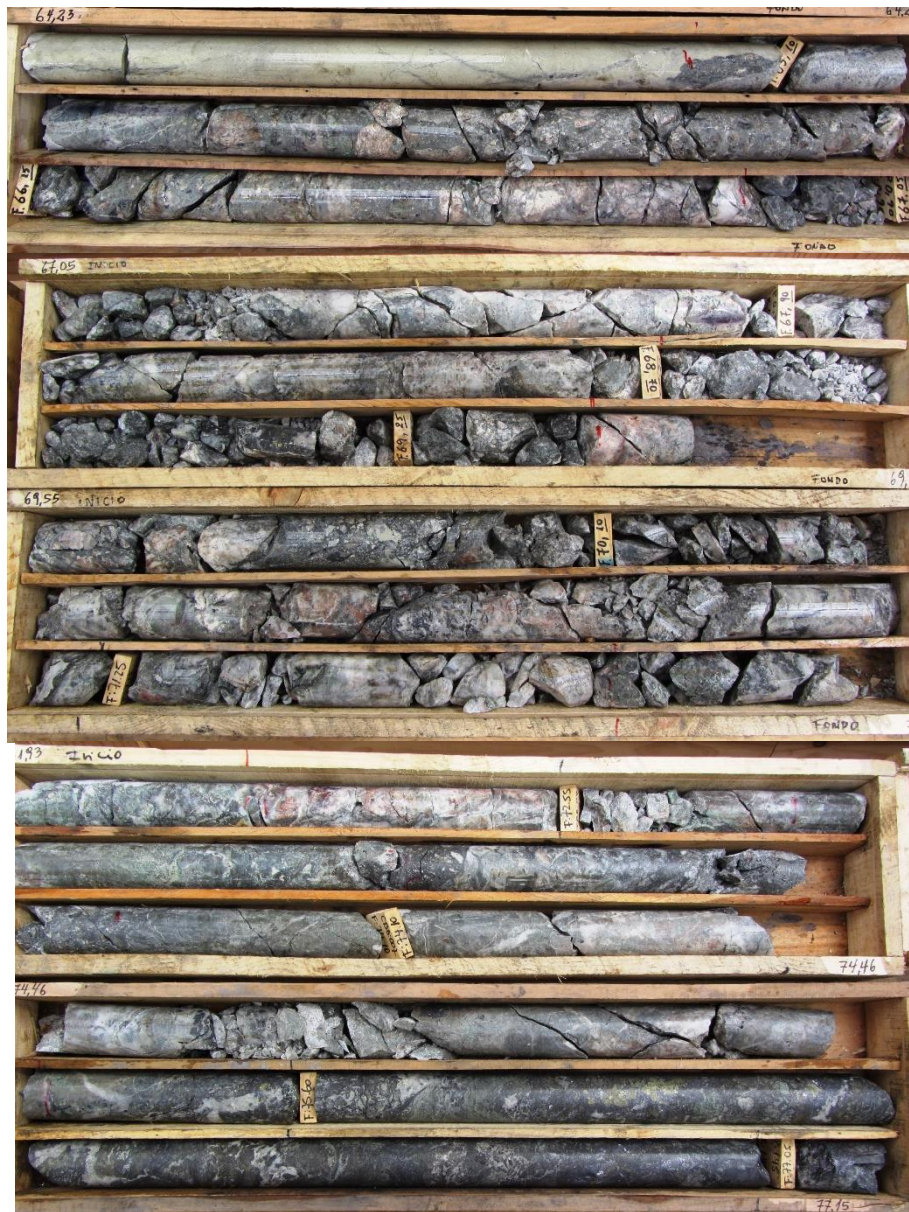
Photo 2. Hole CBD007: 65.05-77.15m interval: Saccharoidal to chalcedonic quartz veining with brecciated vein clasts cemented by black pyrite- Sb-Zn-As-Mo rich chalcedonic quartz
