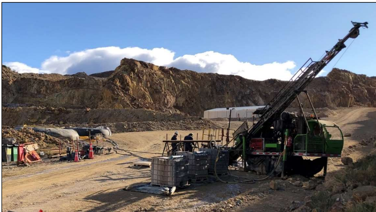
Figure 1 - Cerro Bayo Project - Diamond Drilling within the historic Taitao Pit
