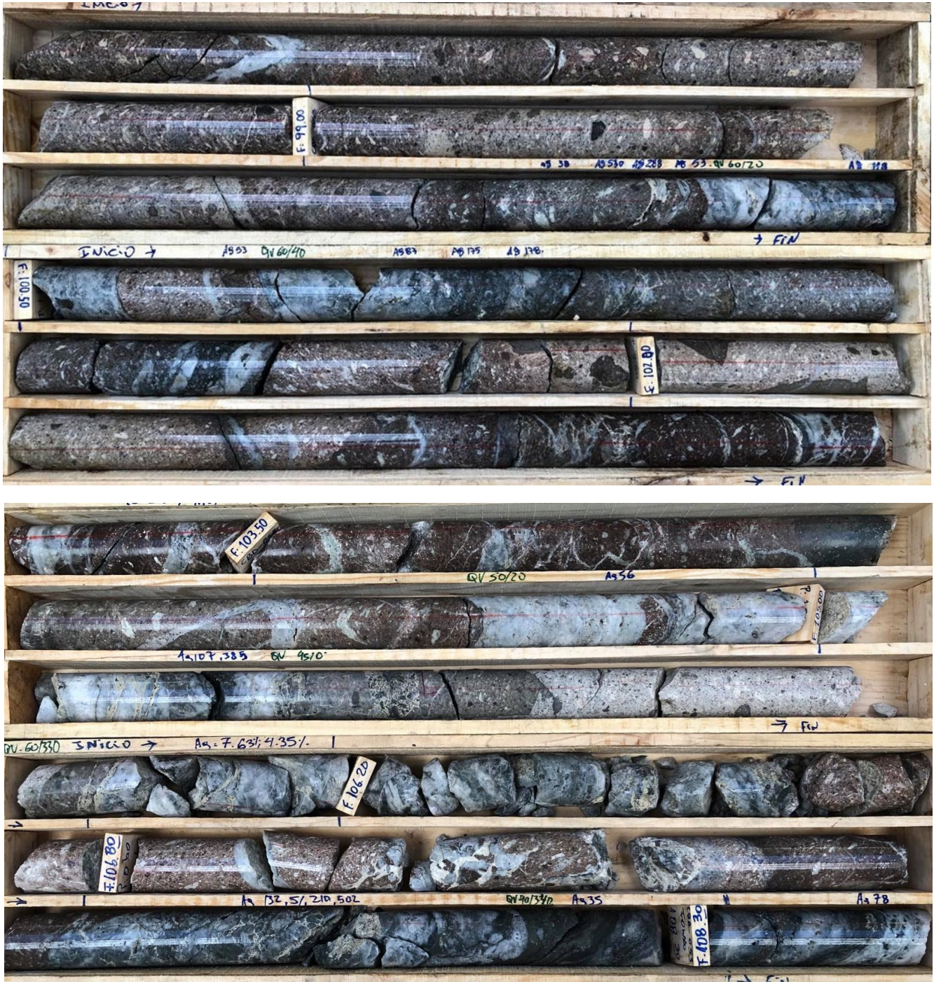
Photo 1: CBD053- example of chalcedonic banded white and crystalline-grey quartz veins between 100.2m to 108.6m for which results are pending
