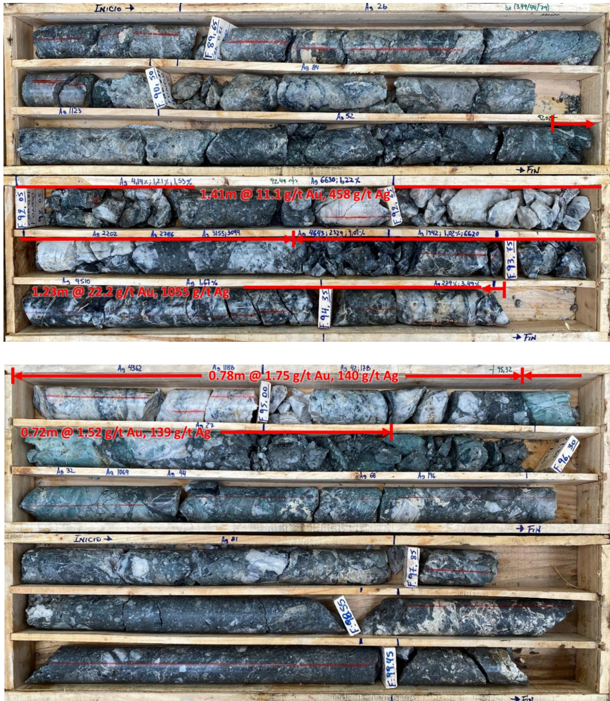
Photo 1. CBD082 drill core displaying the high grade epithermal vein-breccia interval which returned 4.14m @ 11.0 g/t Au, 520.0 g/t Ag (17.9 g/t Au eq 4 ) from 92.01m -96.15m including 2.64m @ 16.3 g/t Au, 736.1 g/t Ag (26.1 g/t Au eq 4 ) from 92.01-94.65m
