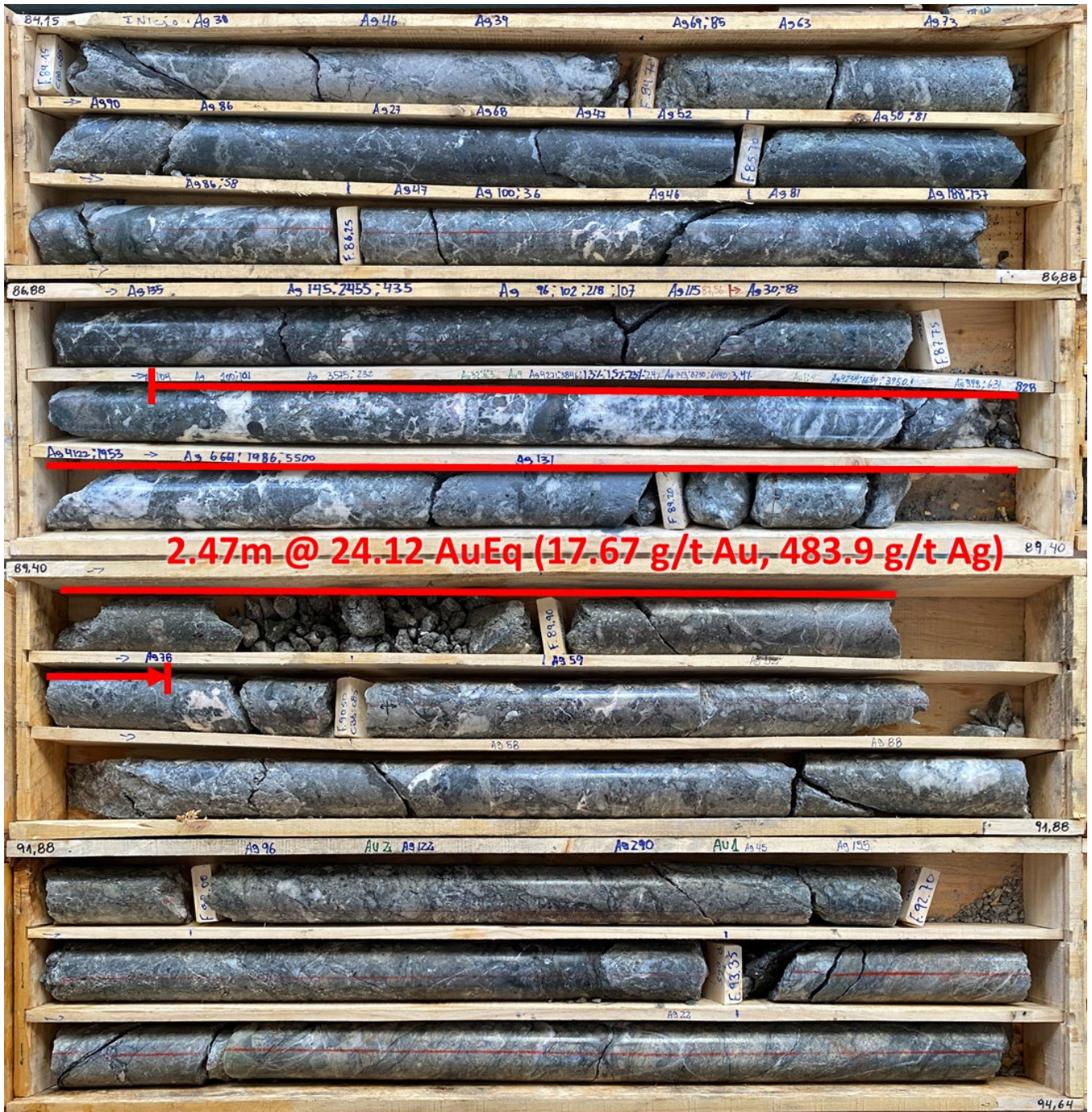
Photo 1. CBD085 drill core displaying the high-grade epithermal vein-breccia interval which returned 2.47m @ 24.1 g/t AuEq 1 (17.7 g/t Au, 483.9 g/t Ag) from 87.87m, within an interval of 7.5m @ 8.7 g/t AuEq 1 (6.0 g/t Au, 206.3 g/t Ag) from 86.08m
