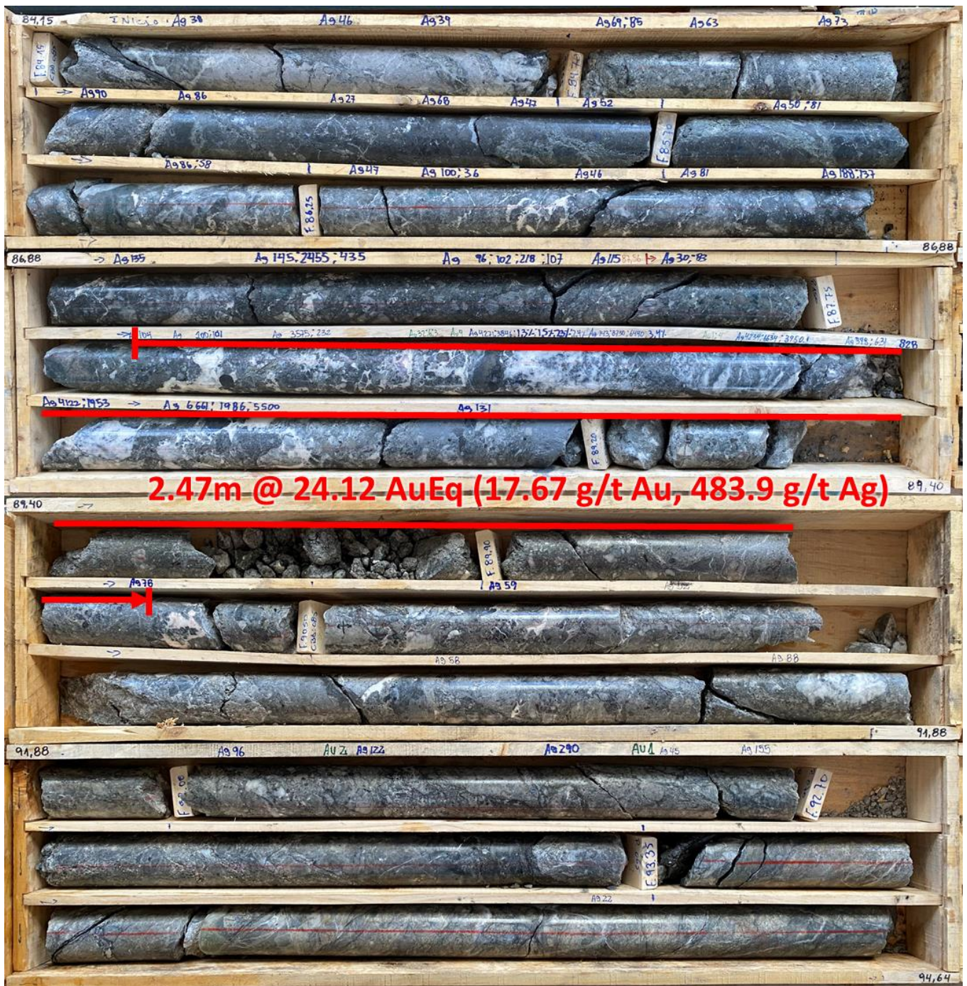
Photo 1. CBD085 drill core displaying the high-grade epithermal vein-breccia interval which returned 2.47m @ 24.1 g/t AuEq (17.7 g/t Au, 483.9 g/t Ag) from 87.87m, within an interval of 7.5m @ 8.7 g/t AuEq (6.0 g/t Au, 206.3 g/t Ag) from 86.08m
