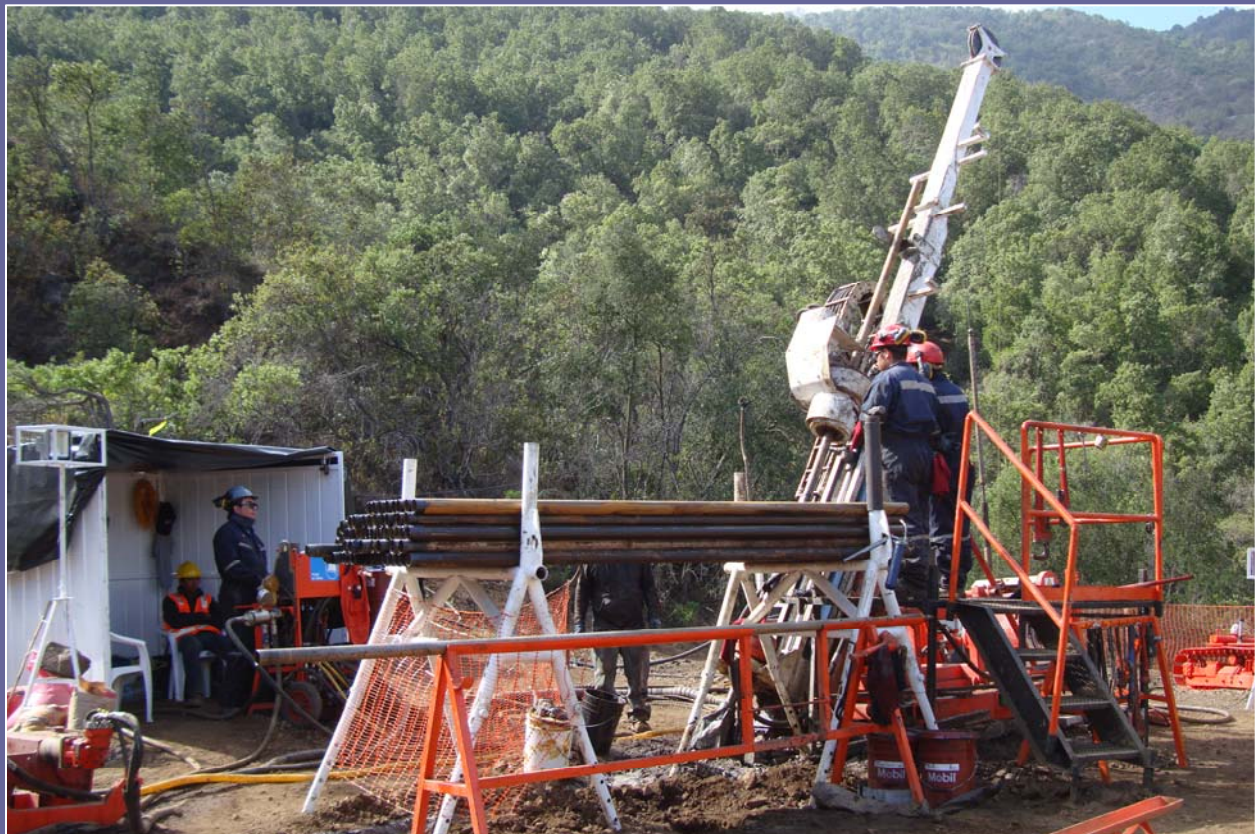
Assad Diamond Rig (1,200m depth capacity - NQ)
