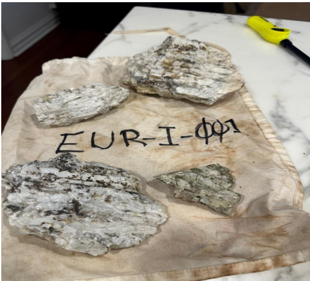
Figure 3 - Coarse grained Spodumene with 3.1% Li 2 O sampled by the previous owner April 2024 from Tenement PL 1597 Knockneen (See EUR Announcement April 2024)
