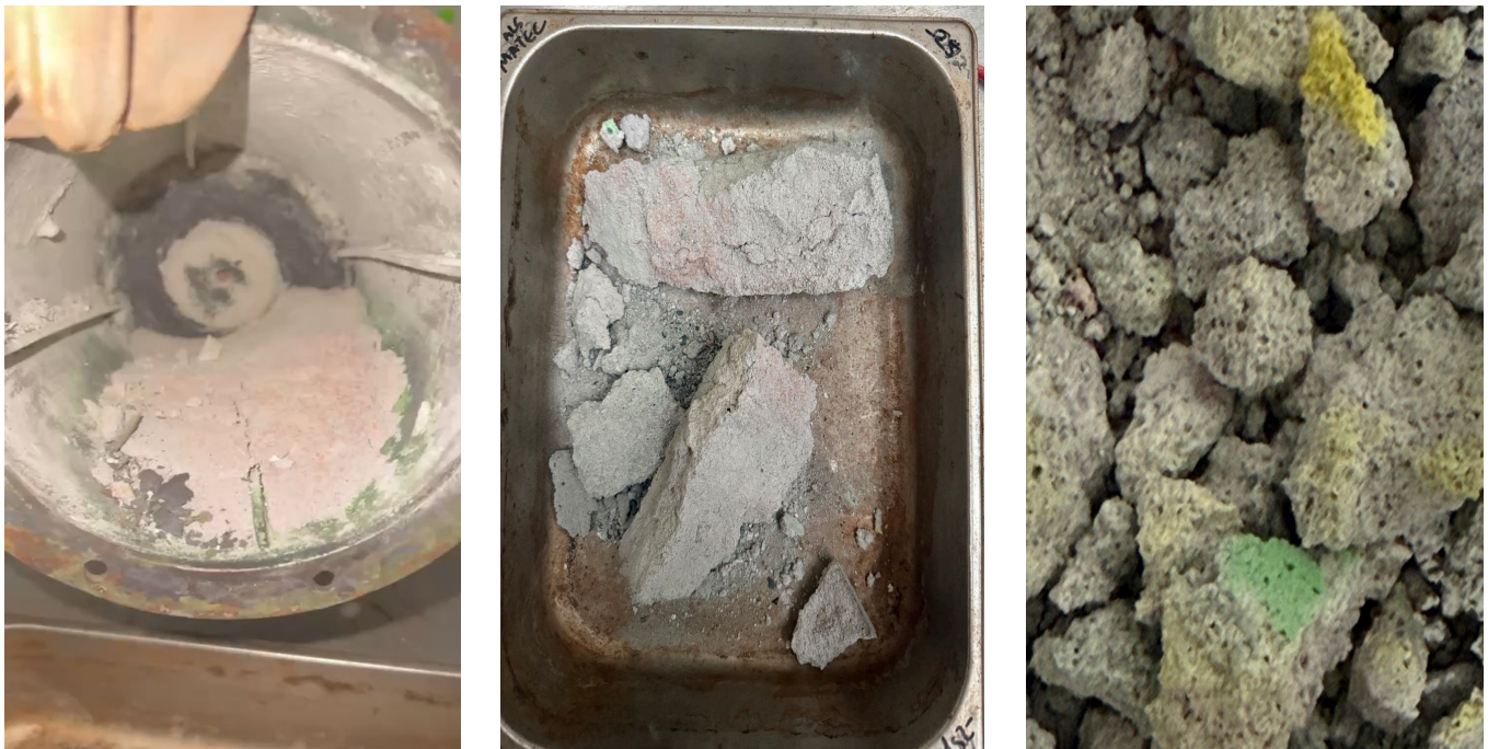
Figure 1: Images of the roasted ore sample (500 g) after static roasting, showing successful processing.
