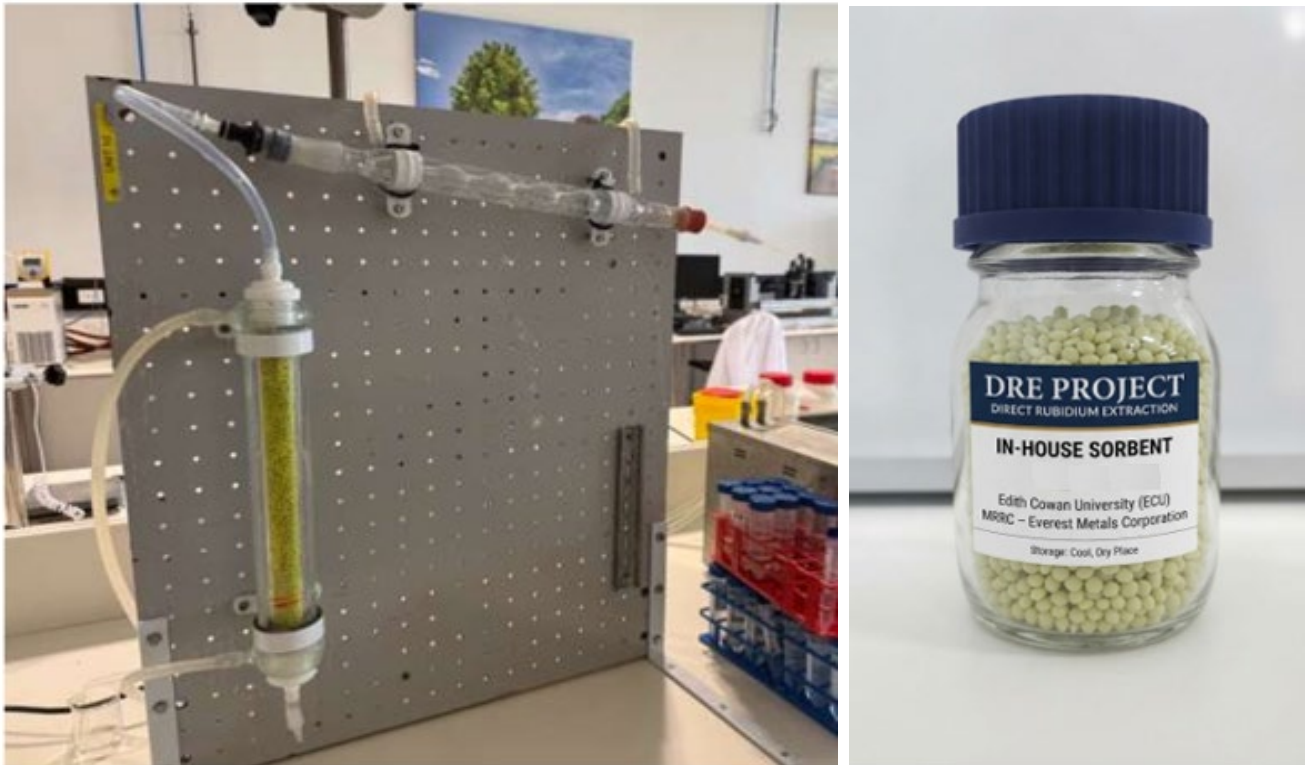
Figure 3: DRE column and the in-house developed DRE Medium used for concentrating and purifying Rubidium
