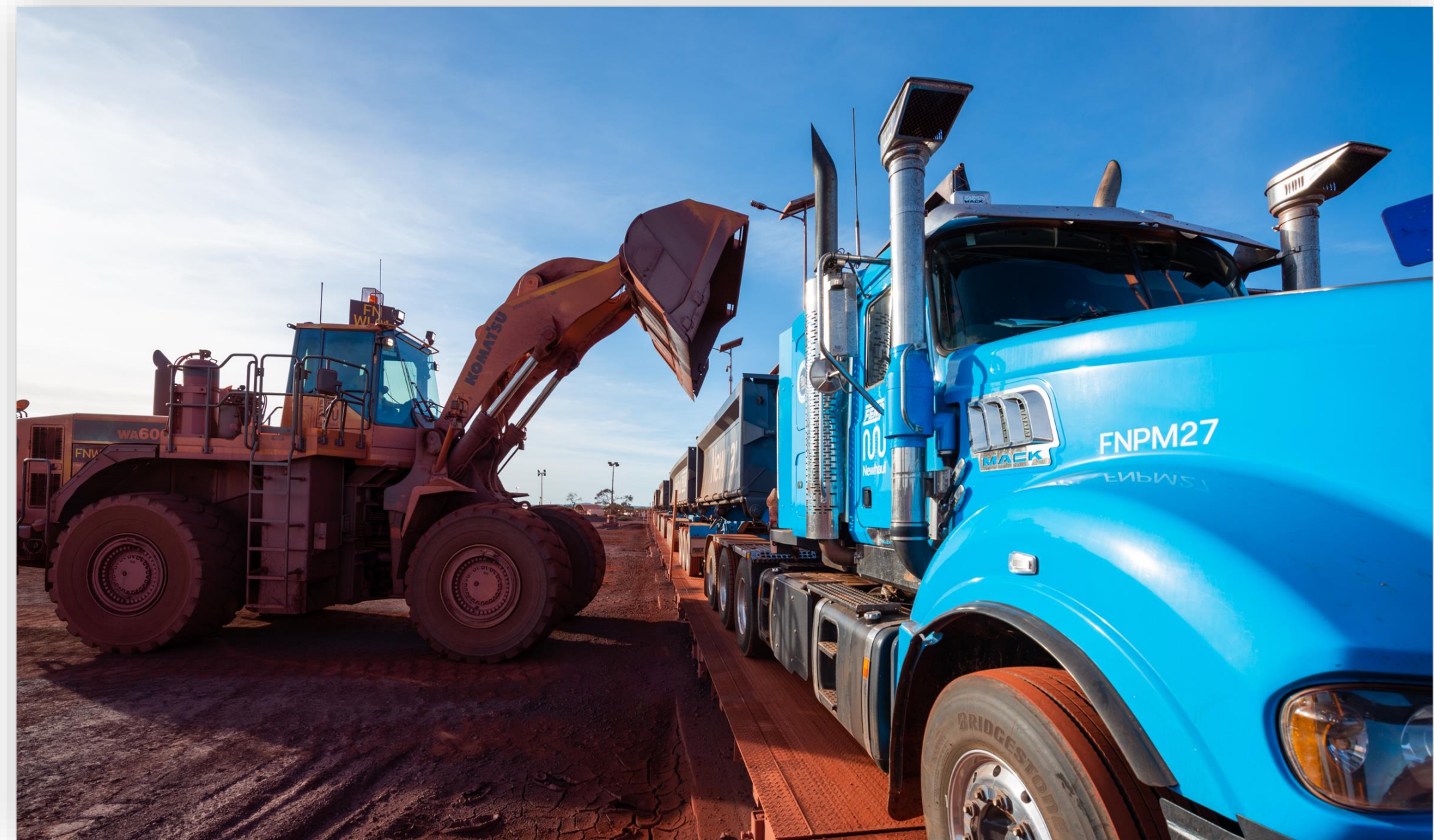
Fenix-Newhaul fleet includes 30 x 200-tonne quad road trains, transporting product from Iron Ridge Mine to Geraldton Port
