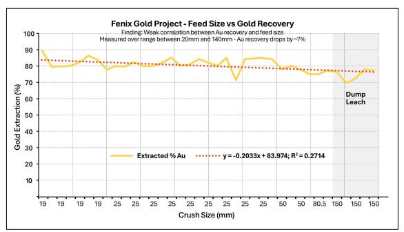
Figure 3: Fenix Testwork - Feed size vs Au recovery
