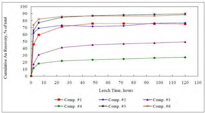
**Figure 13-1**: Gold Leach Rate Profiles, Bottle Roll Test, Pantanillo Drill Core Composites, Nominal 1.7mm Feed Size (Source: McClelland, Nov. 2010)
