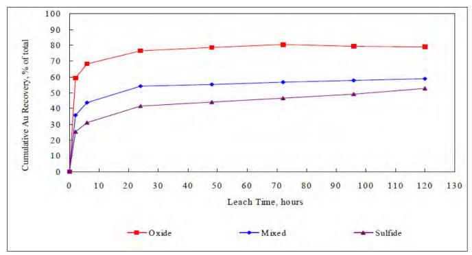
**Figure 13-2**: Gold Leach Rate Profiles, Bottle Roll Test, Pantanillo Composites, 80% - 1.7mm Feed Size (Source: McClelland, Nov. 2010)
