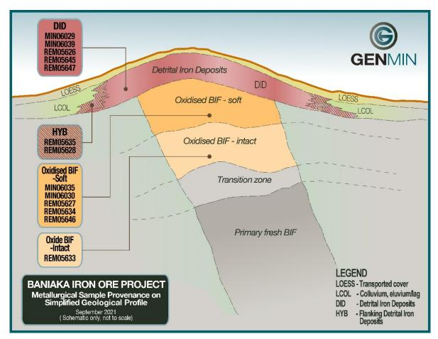
Figure 3: Schematic cross section of Baniaka iron ore mineralisation, also showing respective mineralisation zones for bulk sample selection
