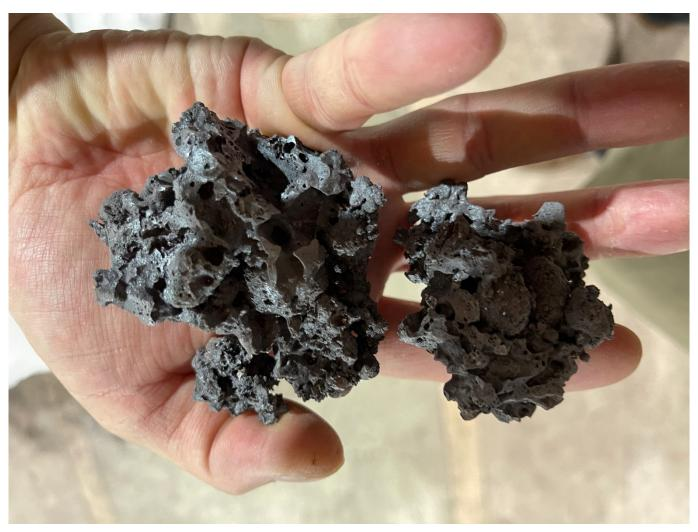
Figure 7: Sinter produced from Baniaka Fines in small pot tests
