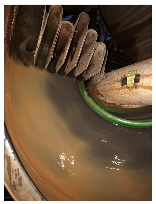
Figure 5: Rougher spiral separation showing iron concentrate on the inside and gangue on the outside
