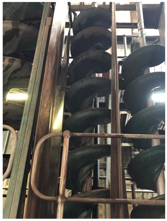
Figure 4: Spiral test rig used by Bond Equipment during the pilot scale test work program
