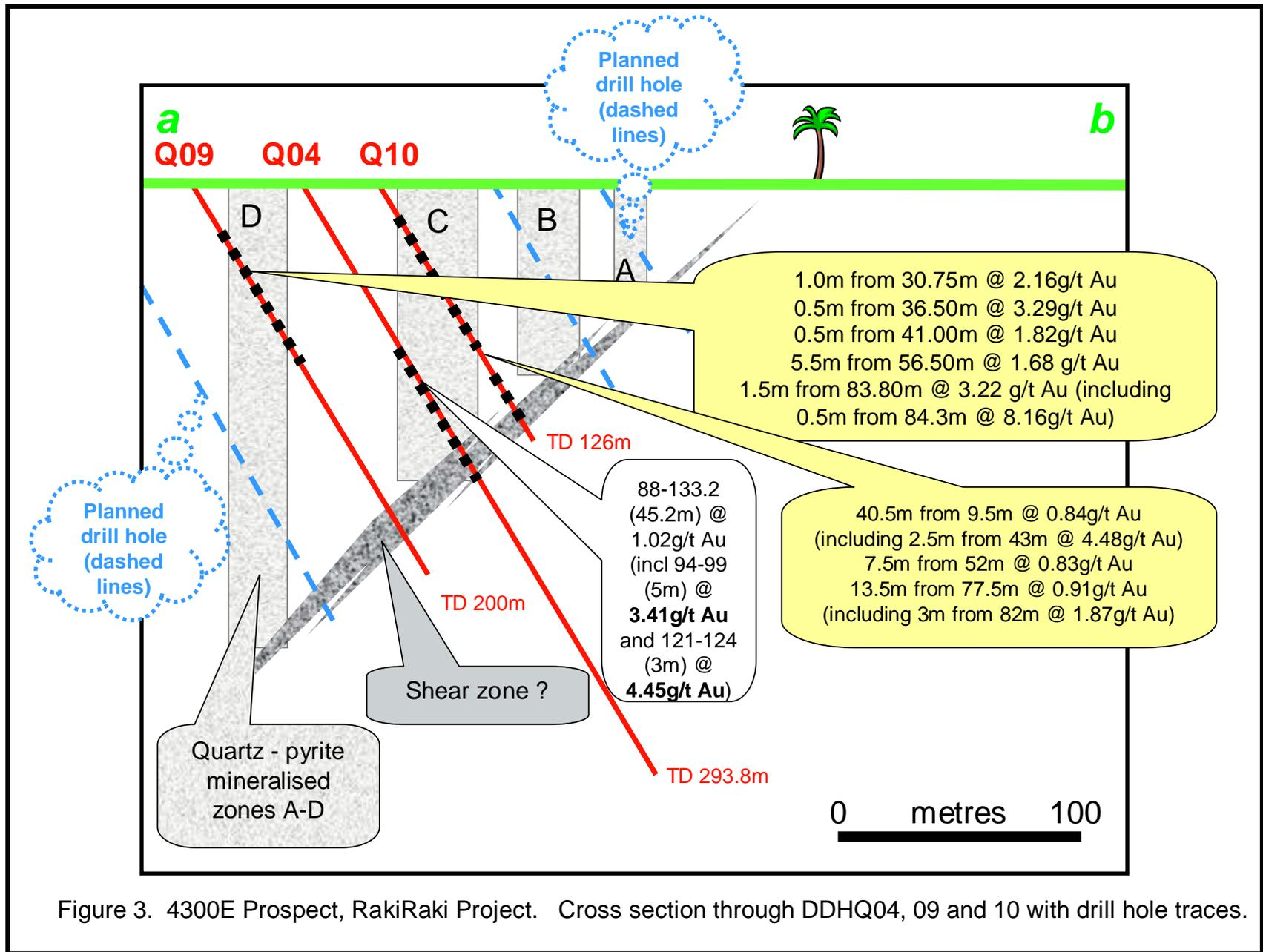
Figure 3. 4300E Prospect, RakiRaki Project. Cross section through DDHQ04, 09 and 10 with drill hole traces.
