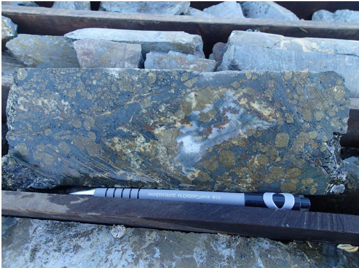
Figure 3 - Semi massive sulphide DH 100-1-H, 36.6m, interval assay , 2.77% Cu, 0.05 g/t Au, 0.02% Zn
