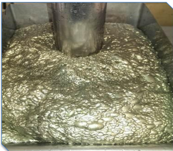
Figure 9 Chalcopyrite and telluride in froth in laboratory flotation cell
