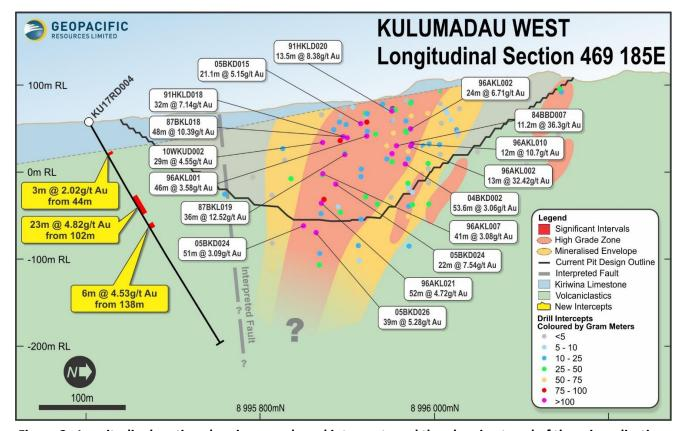
Figure 2: Longitudinal section showing new, broad intercepts and the plunging trend of the mineralisation.
