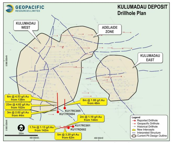
Figure 1: Drillhole location plan showing the drillholes for current results (bold red) and in relation to current pit designs at the Kulumadau deposit. Drill holes with assays pending are shown in light red.
