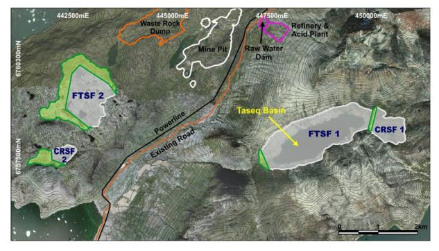
Figure 8. Overview of the Kvanefjeld Project area, showing the location of the two proposed tailings storage facility locations. Tailings Storage Facility scenario 1, located in the Taseq basin, is the preferred option.
