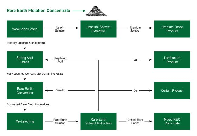
Figure 7. Metallurgical design of the refinery circuit.
