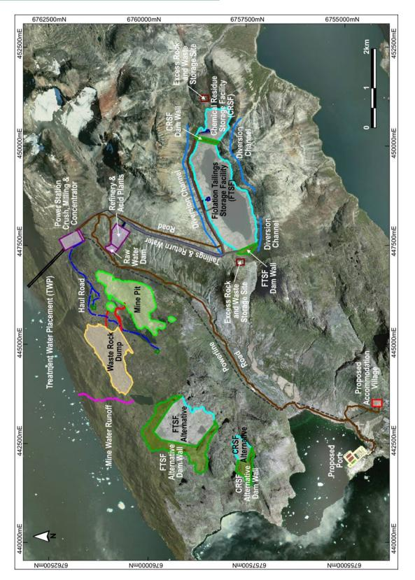
Figure 12. Overview of the Kvanefjeld Project and surrounding areas, highlighting the infrastructure requirements for the project.
