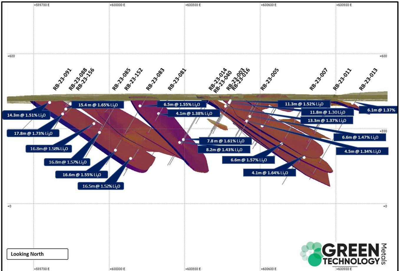
Figure 4: Root Bay stacked pegmatites looking north
