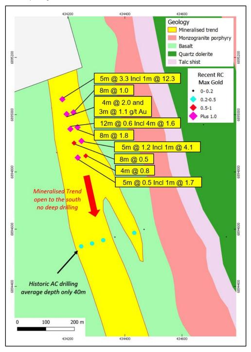
Figure 4 – Gold drilling results at Golden Boulder.
