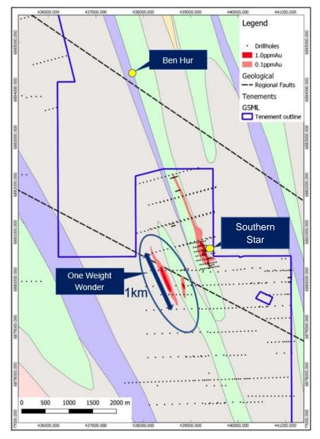
Figure 3 - Plan view of historic RAB holes highlighting the very limited exploration undertaken at the One Weight Wonder target.
