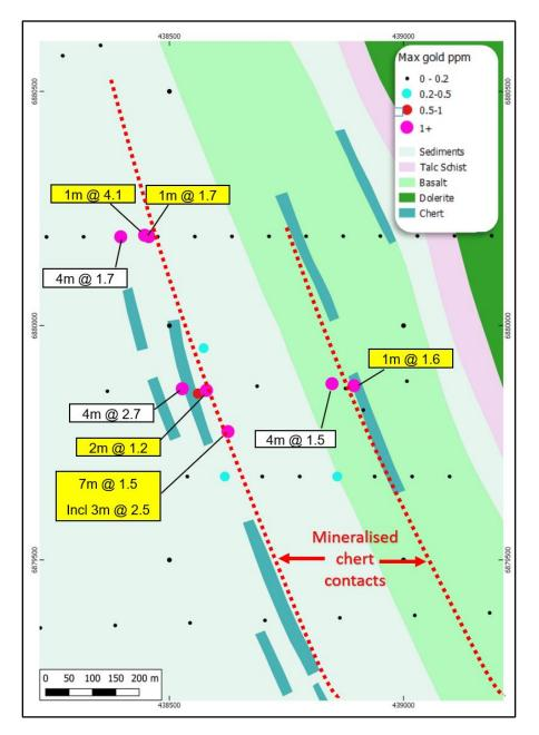
Figure 2 - Plan view of One Weight Wonder highlighting recent significant drill intersections (yellow) and anomalous historic RAB intersections.
