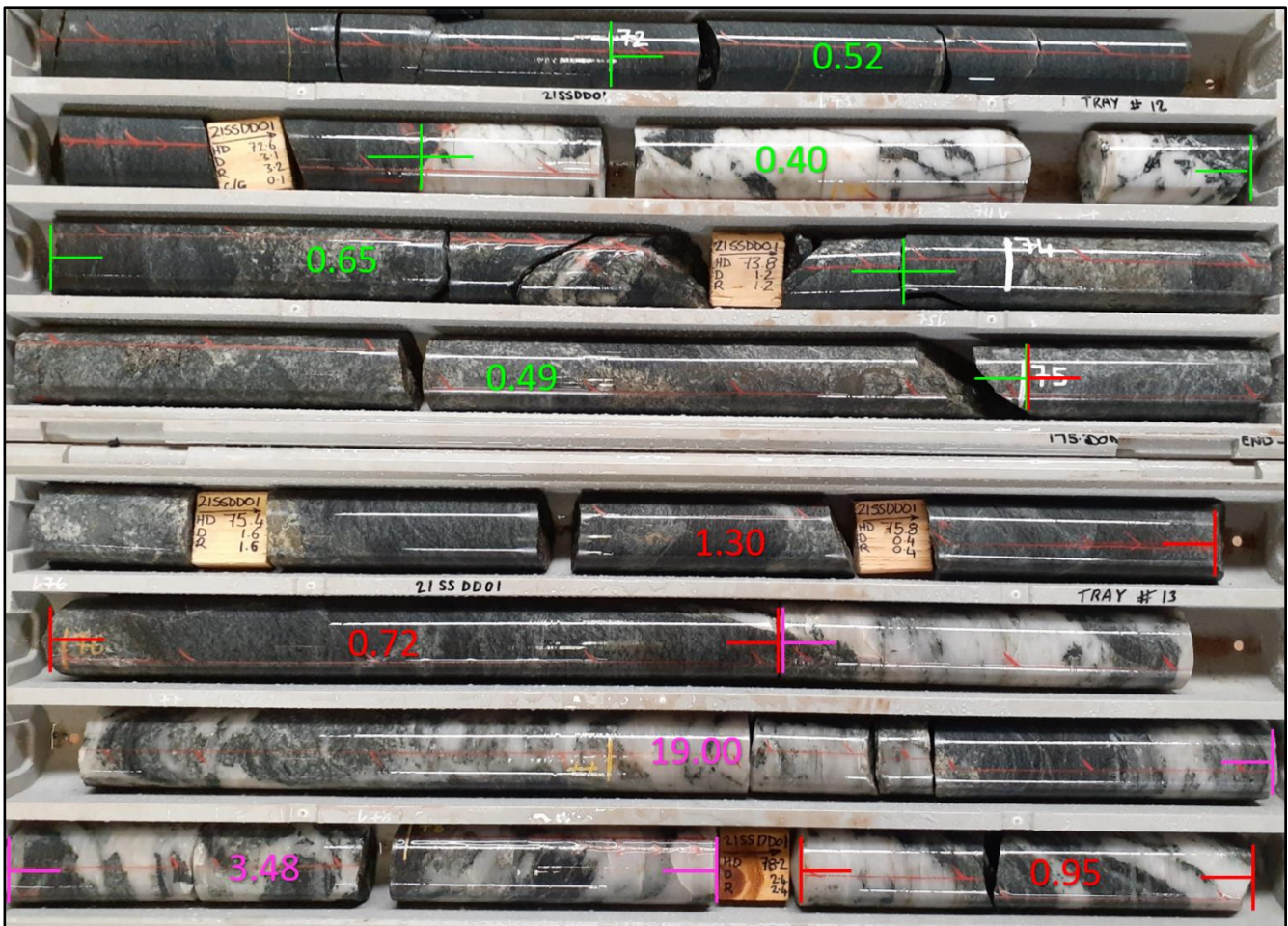
Figure 4 - Diamond Core photo of 21SSDD001, highlighting high grade gold intervals (g/t Au) from 72m-78.4m with intense albite alteration overprinting and hydrothermal veining.
