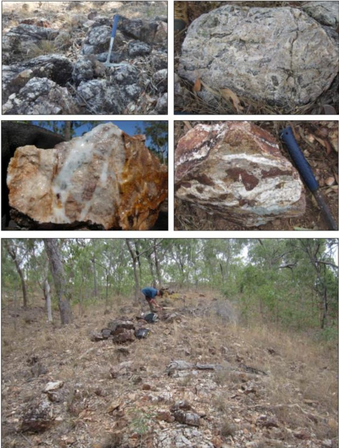
Figure 4: Examples of epithermal mineralisation in outcrop and rock chip sample from the Whydah Prospect
