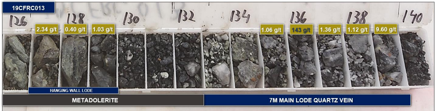
Figure 1: Cox's Find Project: High grade quartz lode (Main Lode) intersected in 19CFRC013 (RC chip sample tray)
