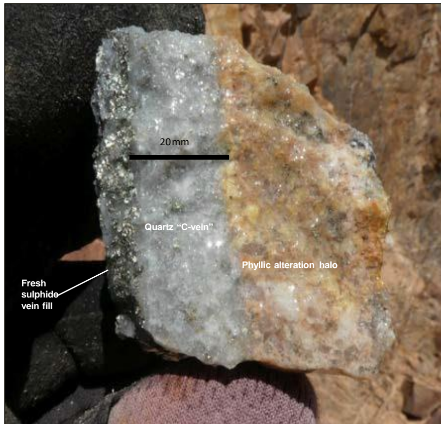
Transition through sulphide vein fill central to the quartz vein and strong phyllic alteration halo.
