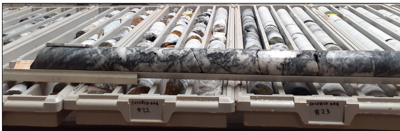
Figure 1: Intersection 164.6 to 165.8m (above) highlighting the interpreted Cox's Find main lode with close up photos (below) of visible gold identified at 164.5m.
