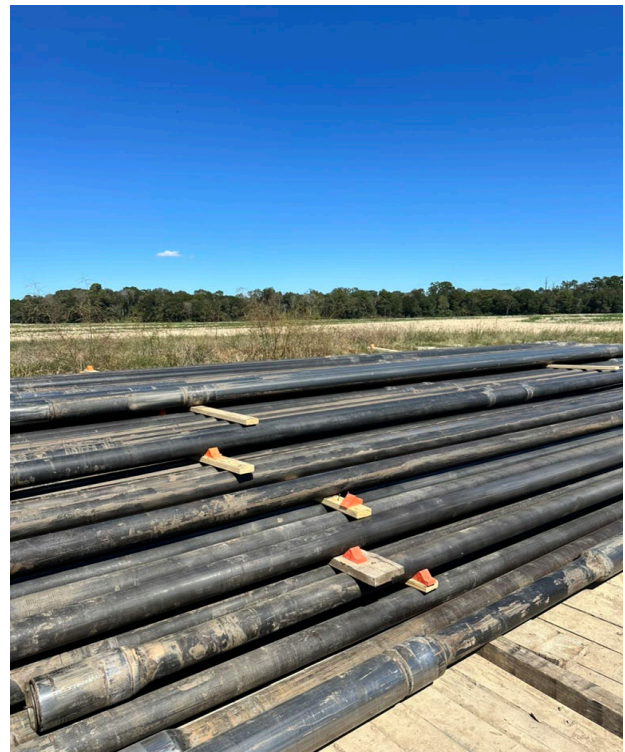
Figure 5: Tubulars stored on racks at the well site.
