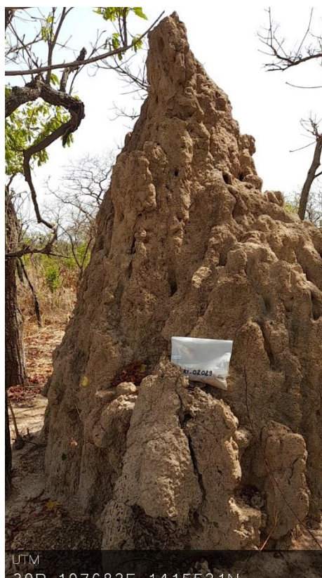
Figure 1: Typical "cathedral" termite mound in the Saraya permit area. Termites build their mounds with material from up to 30 metres below the surface. Surface sampling of the termite mounds can therefore detect uranium mineralisation in the bedrock below thick saprolite cover.
