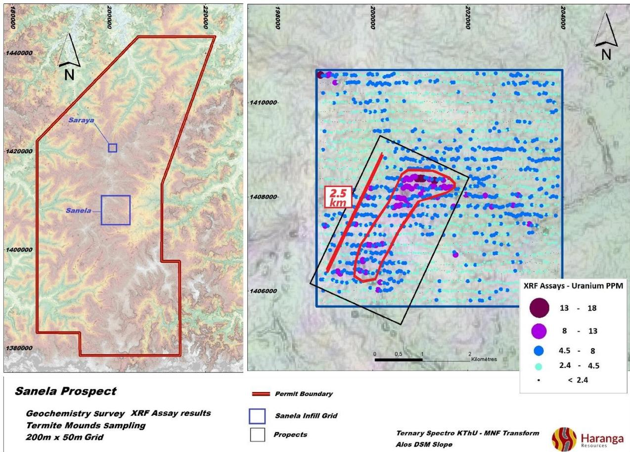
**Figure 2: Uranium results for the termite mound infill sampling over the Sanela Block. The results outlined a large uranium anomaly, fifteen kilometres South of the Saraya Maiden Resource. All analysis was carried out using an in-house XRF analyser.**
