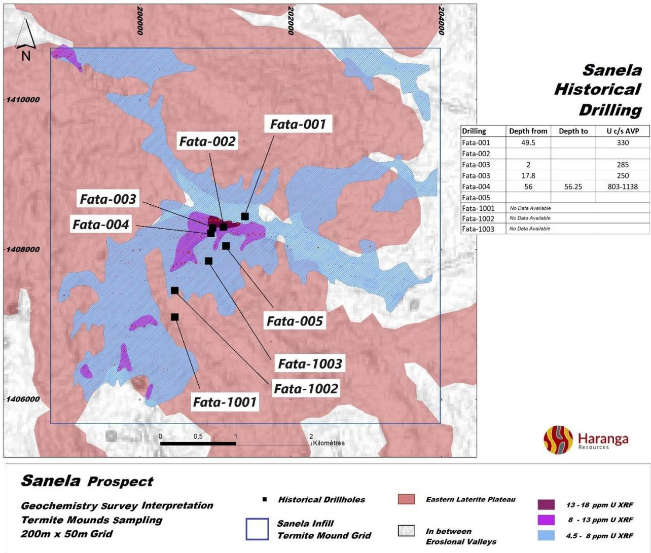
Figure 3: Interpretation of termite mound infill sampling results for the Sanela Block. The uranium anomaly detected is located along a NNE trend of +2km long.
