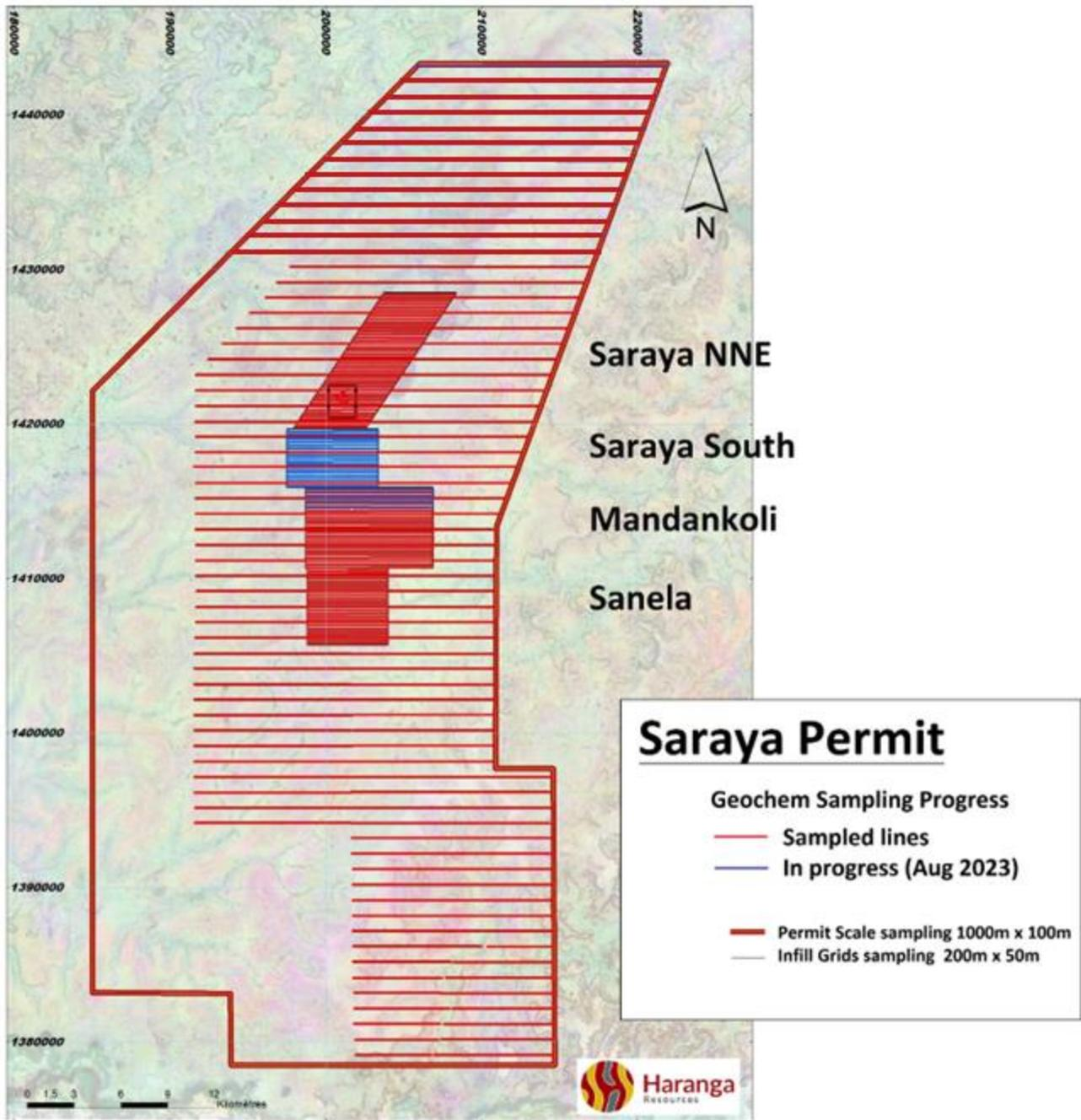
Figure 4: Termite mound sampling progress to date: Red lines show the sampled lines, while blue lines show the remaining program to be completed. A total of +70% of the permit surface has been covered by the 1000m x 100m sampling survey. The three first Infill grids (200m x 50m) defined in the central area of the permit have been completed and the fourth grid (Saraya South) will be completed by the end of the year.
