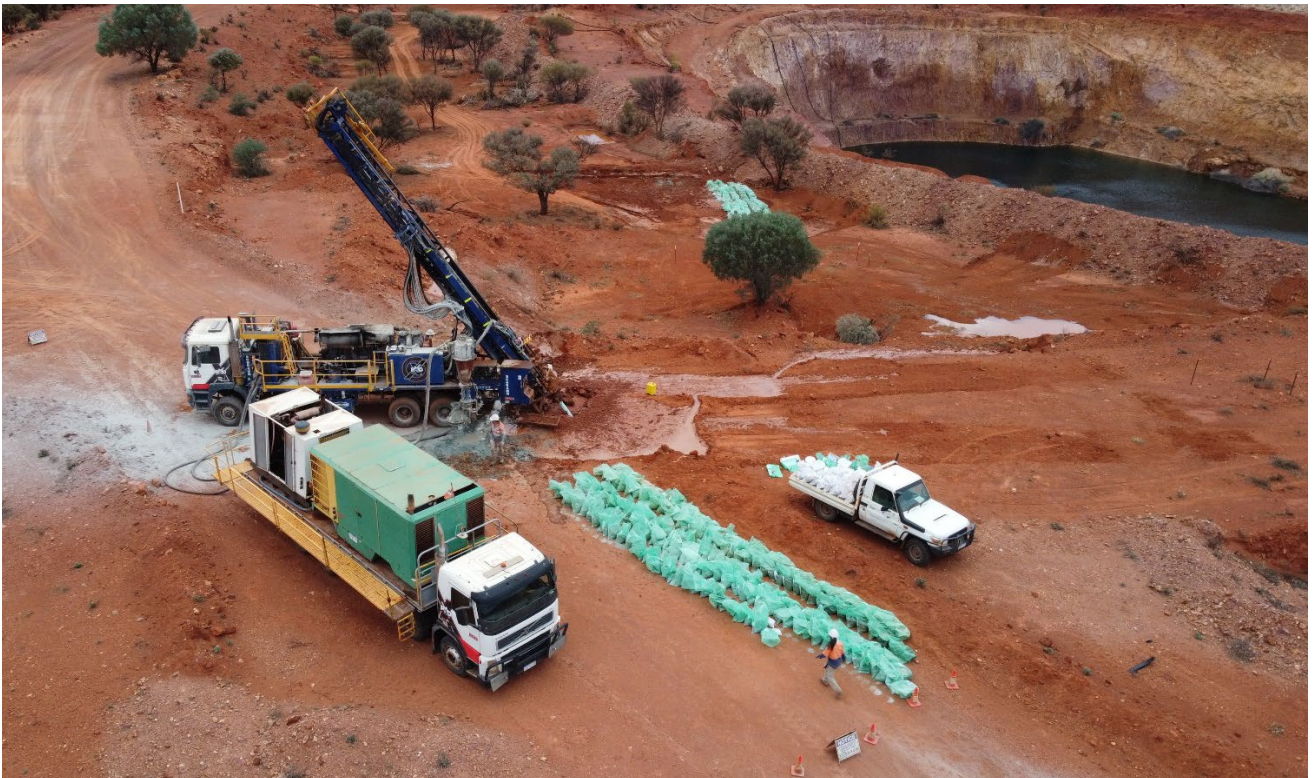
FIGURE 3: RC DRILLING AT THE EAGLE PROSPECT
