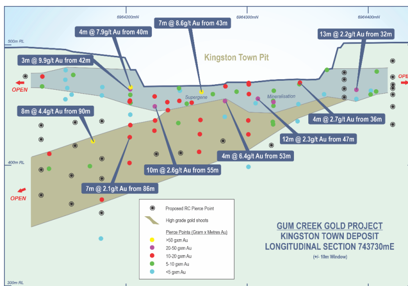
Figure 8: Kingston Town long section showing interpreted high-grade ore shoots and planned drilling mineralisation pierce points.
