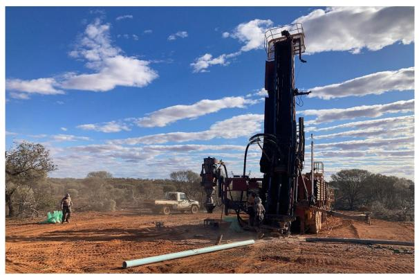
Figure 2: RC drilling at the Mensa Prospect.
