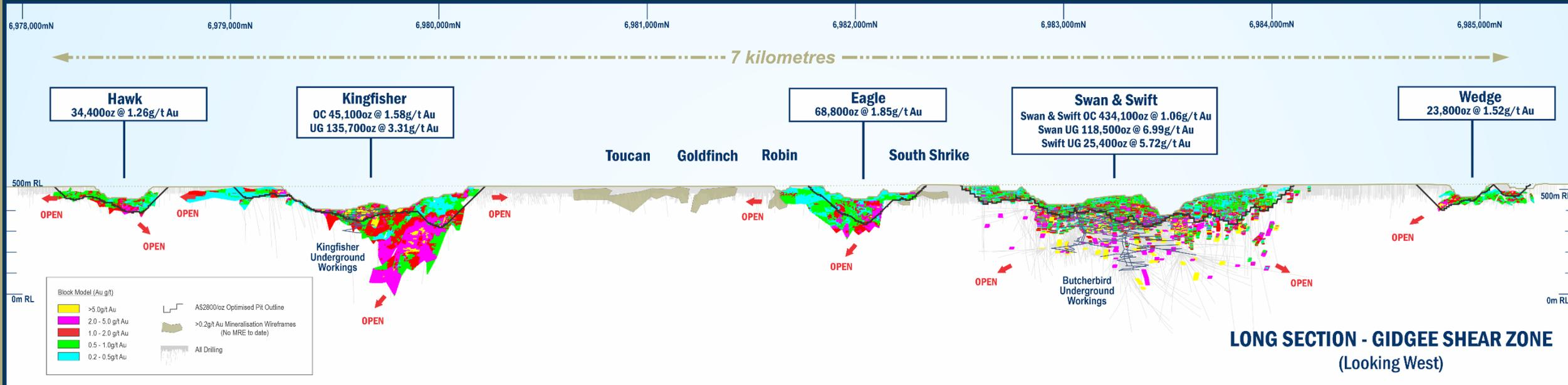
Long Section showing all drill traces, existing pits, \$2800/oz optimised pit shells, >0.2g/t Au mineralisation & resource block models coloured by Au (g/t).
