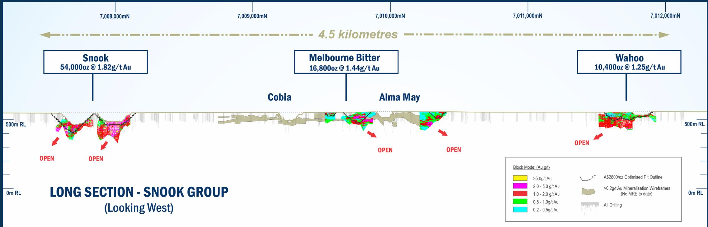
Long Section showing all drill traces, existing pits, \$2800/oz optimised pit shells, >0.2g/t Au mineralisation & resource block models coloured by Au (g/t).
