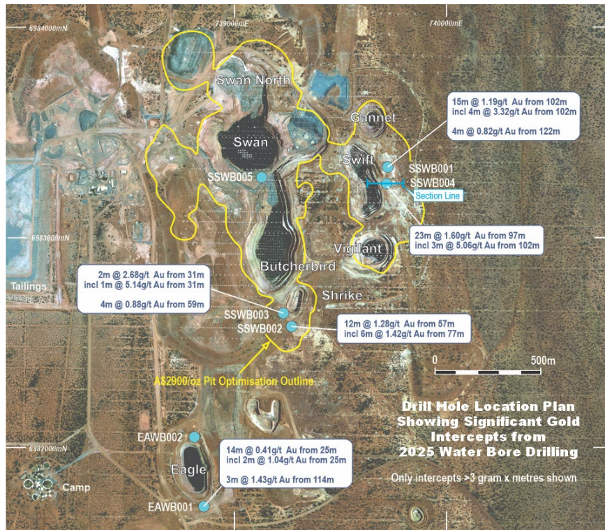
Figure 5: Swan-Swift Area drill hole location plan showing A$2900/oz optimised pit shells outlined, water bore collars (blue) and water bore gold intercepts >3 GxM (labelled) over satellite image.
