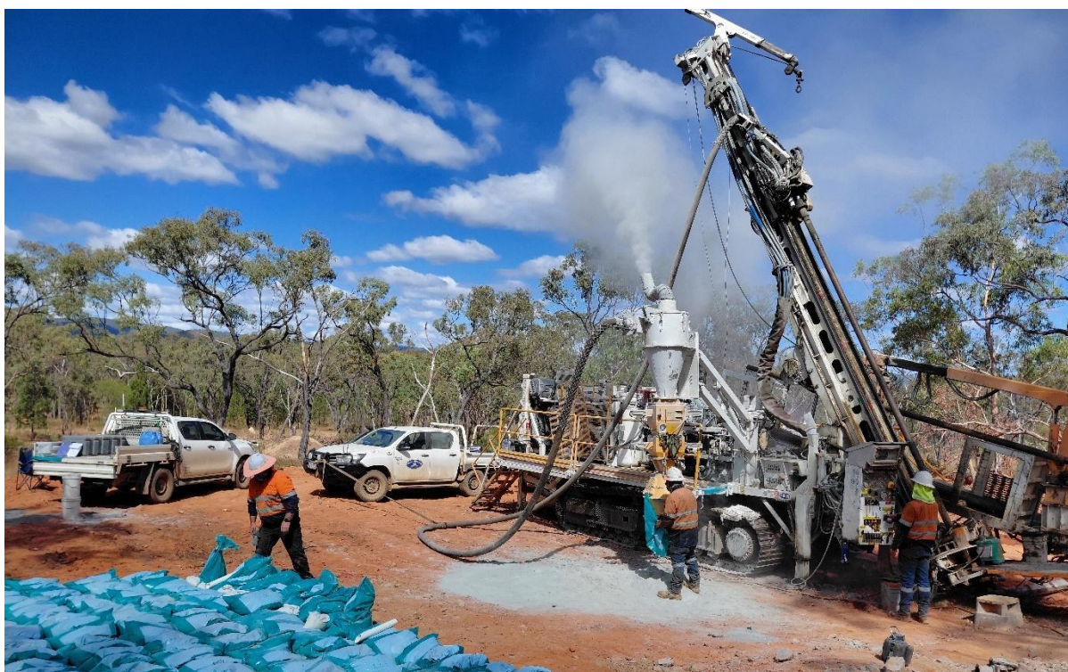
Figure 1 RC drill rig drilling at the Orient Project
