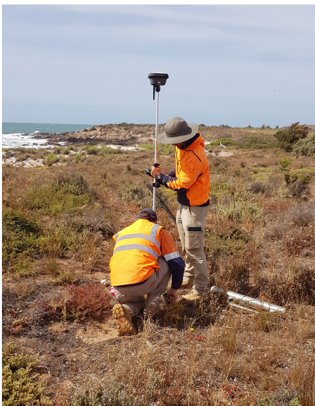
Surveying of control point at Cape Hardy
