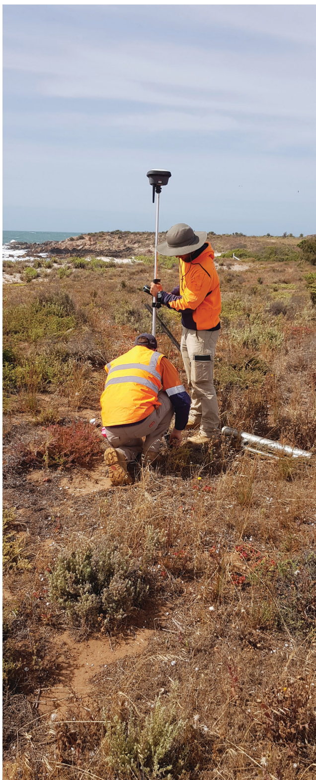
Surveying of control point at Cape Hardy
