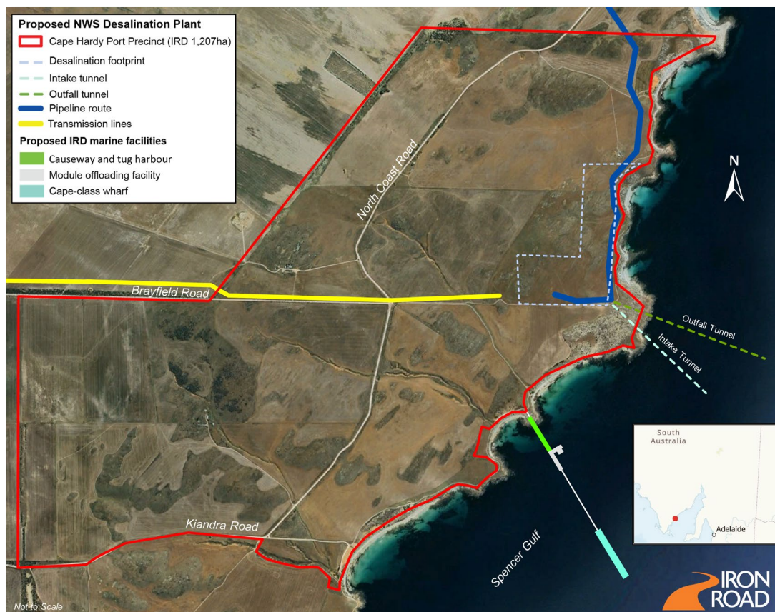
Iron Road and Northern Water Supply (NWS) Cape Hardy Spatial Reference – Preliminary site plan for proposed desalination plant
