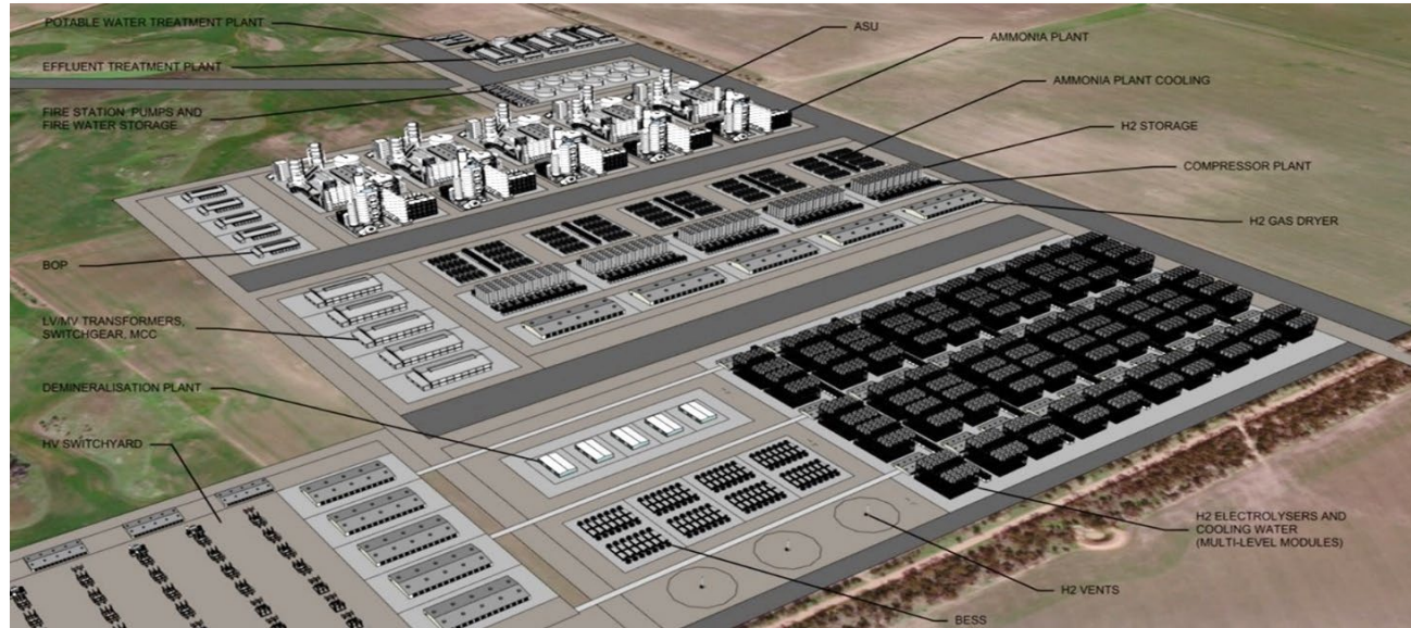
Source: Amp Energy - Key plant building blocks, Cape Hardy 5GW Advanced Fuels project
