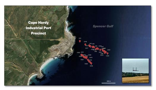
Locality of completed offshore geotechnical drillholes at Cape Hardy, aligning with the proposed intake and outfall tunnels for the proposed Northern Water desalination plant
