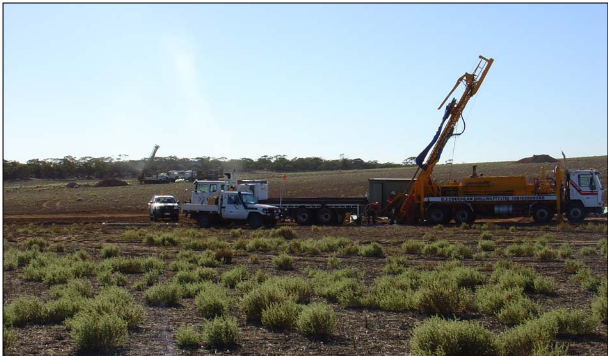
Figure 1 RC drilling (background) and diamond drilling (foreground) at Boo-Loo
